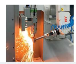
It is the most up-to-date part cutting method where you can cut metals (Stainless, Iron, etc.) in flat plates or 3D pieces, fully automatic parts with a thickness between 0.2mm and 20mm with fiber laser cutting method.
